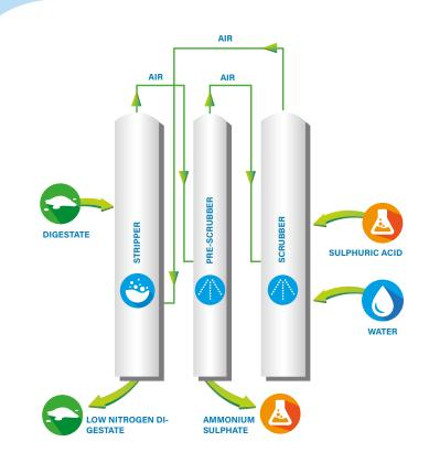
These 2 parameters are vital for the design of the stripper.
